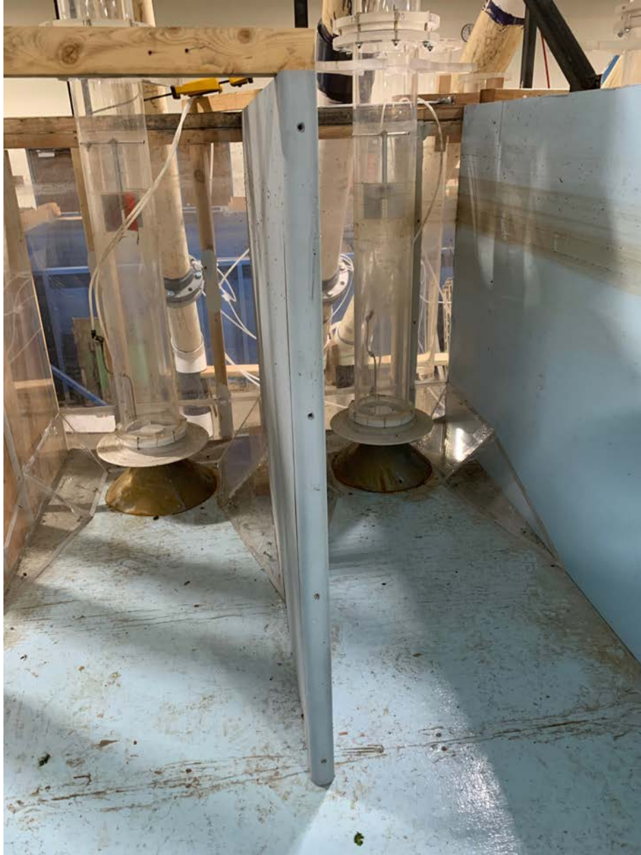
Figure 28. Final fixes in the pump bay containing pumps 8 and 9
