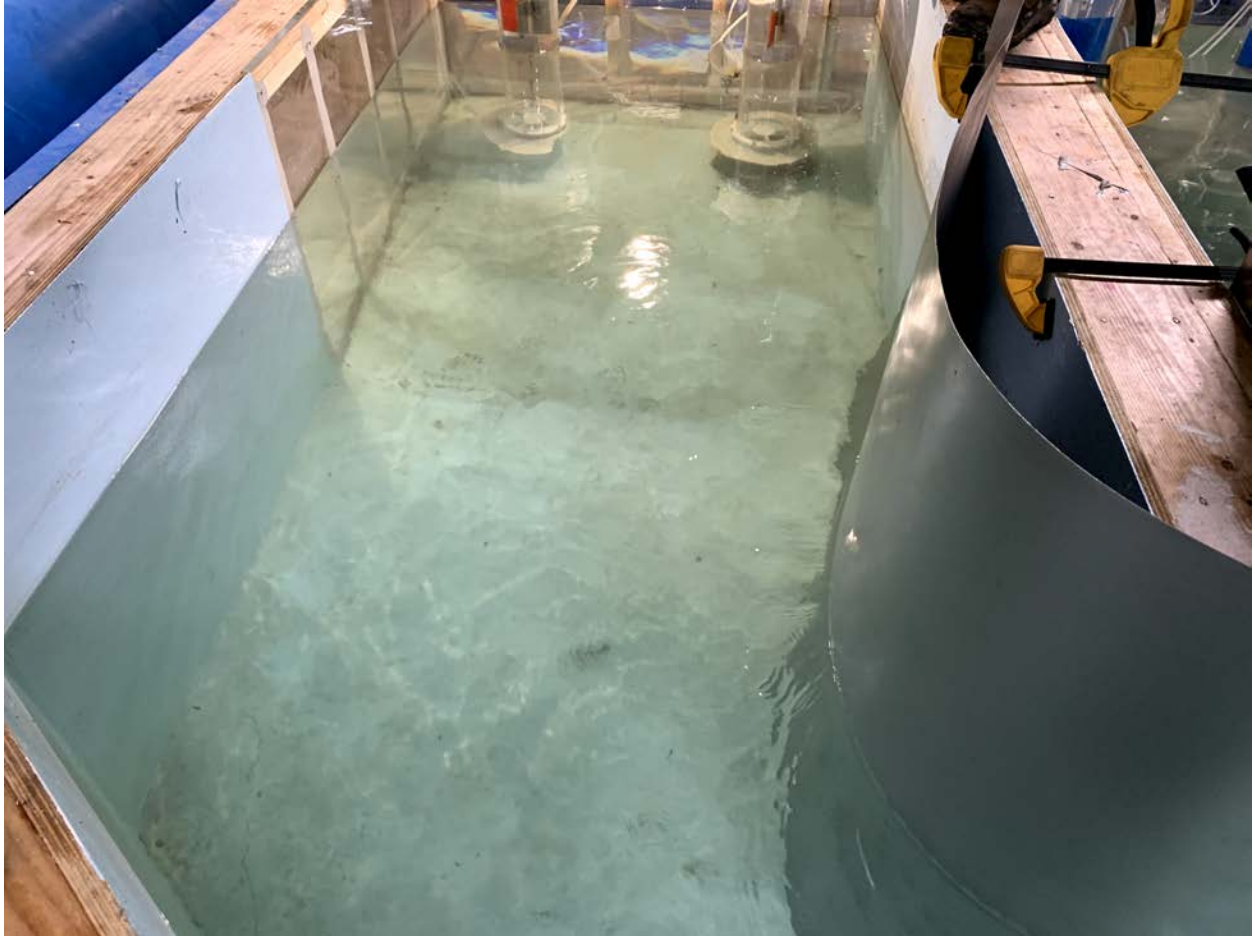
Figure 22. Trial warped nose cone
