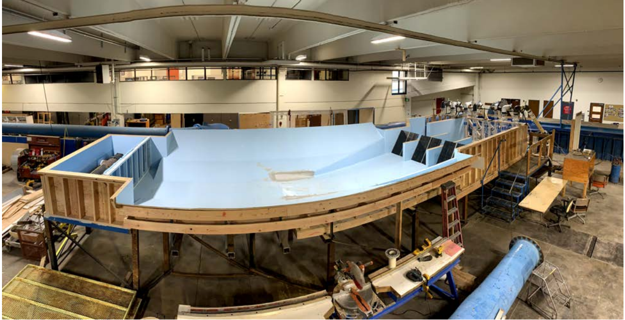
Figure 3. The 1:5.7915 scale physical model of the RD1000 pumping plant
