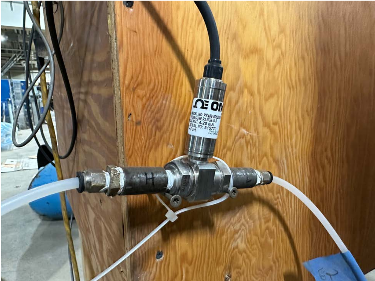
Figure 16. Pressure transducer used to make pitot tube velocity measurements
