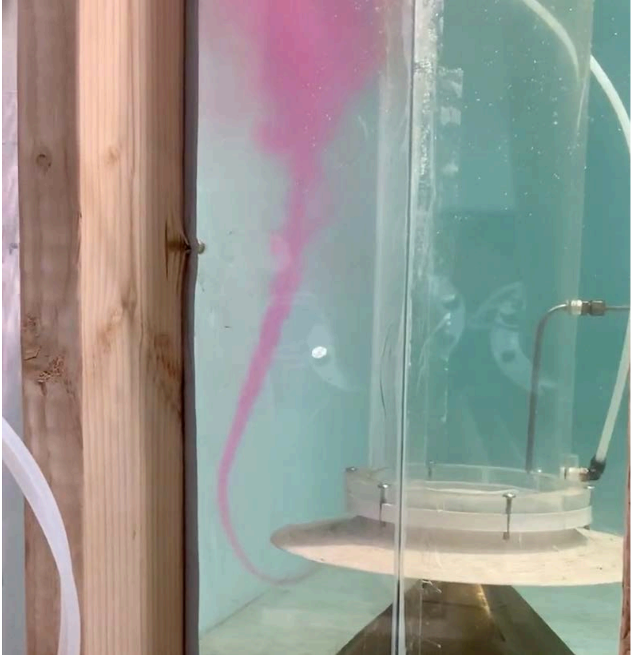
Figure 26. Example of surface vortex in the pump bay containing pumps 8 and 9
