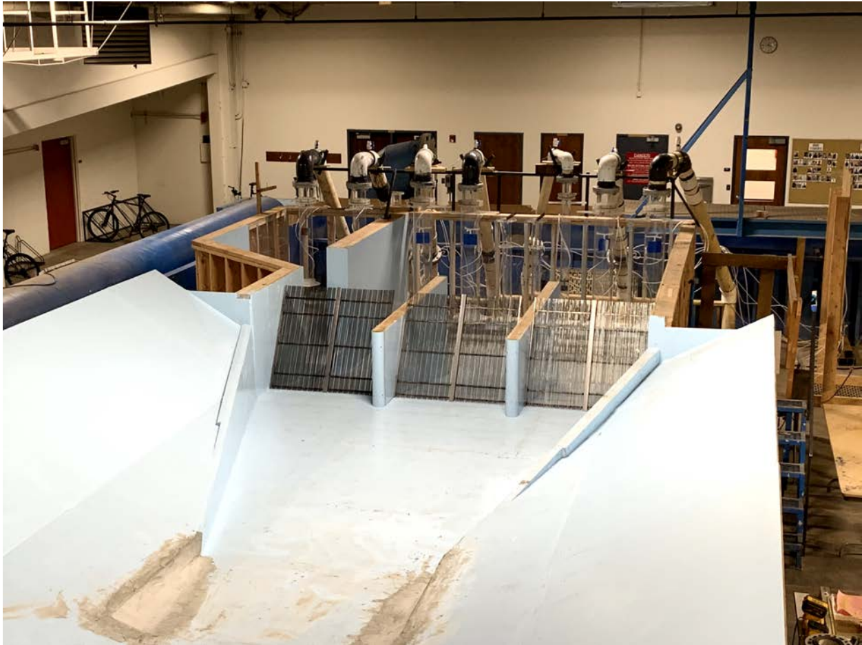
Figure 14. Simulated pump station in the model
