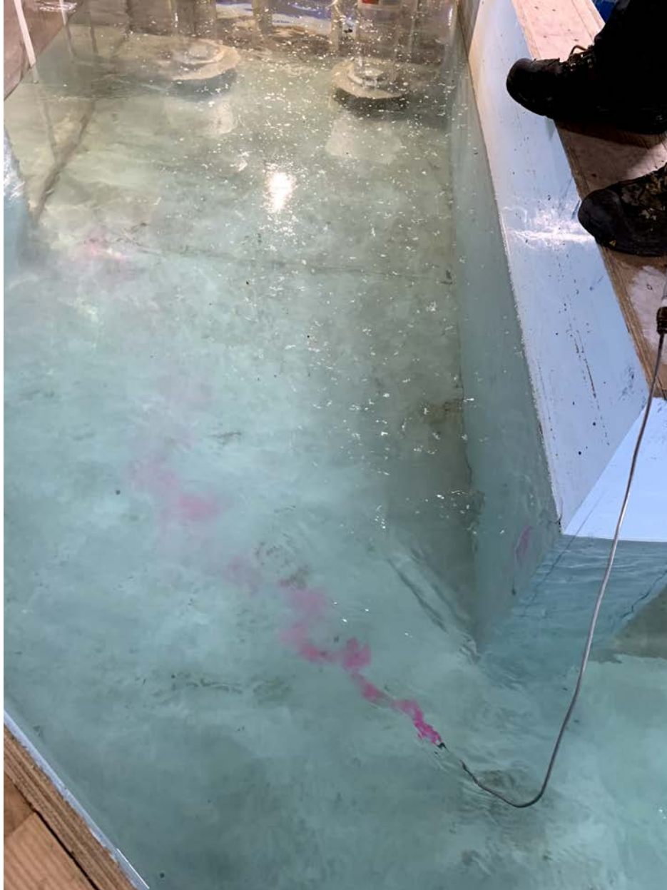
Figure 25. Flow separation entering the pump bay containing pumps 8 and 9
