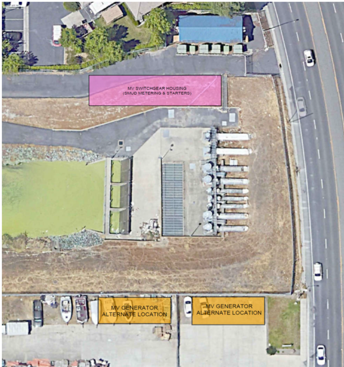
Figure 5-4 Recommended Equipment Location Alternative
