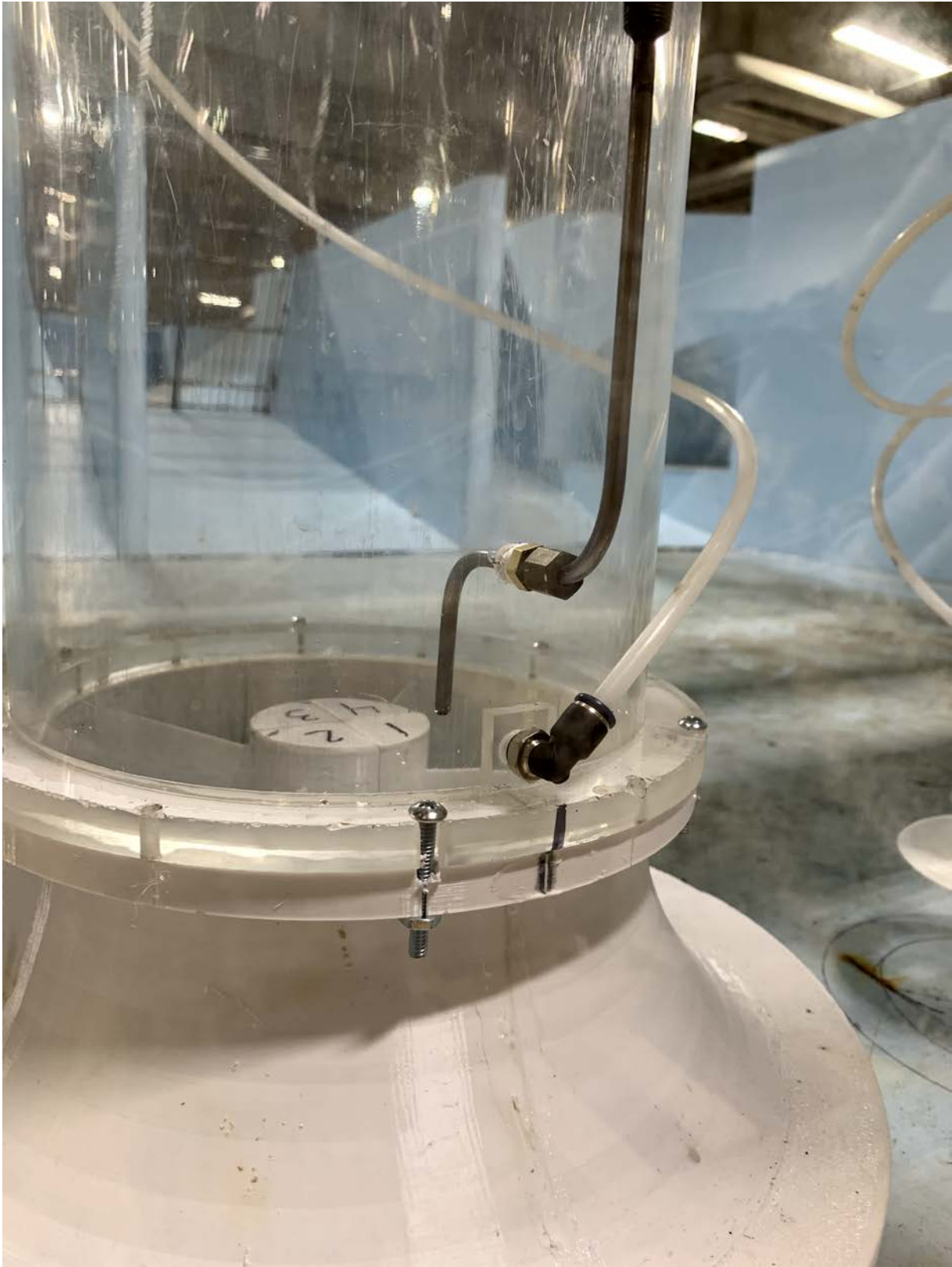
Figure 15. Pitot tube configuration in each pump riser
